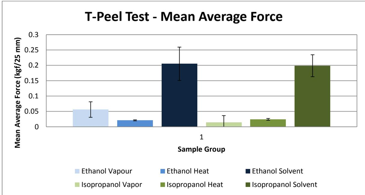
Fig. 9: T-Peel Test- Mean Average Force
