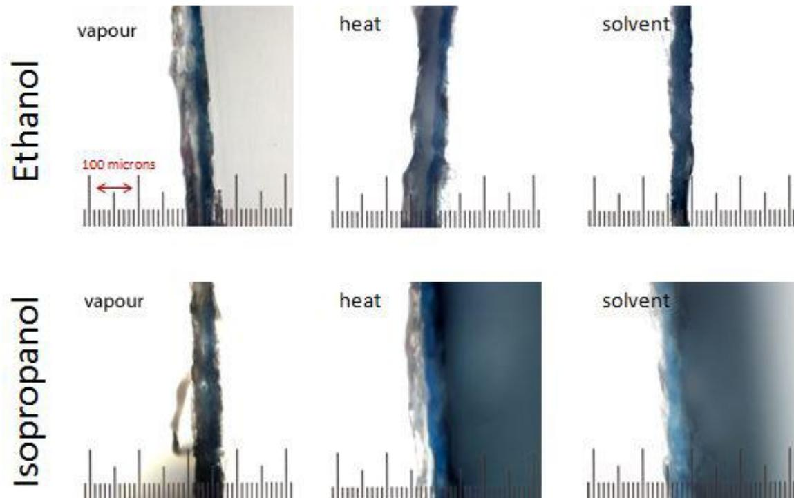
Fig. 10: Photomicrographs of dyed adhesive sample cross sections
