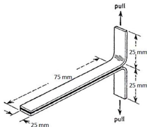
Fig. 7: T-Peel test measurements (ASTM 2008)
