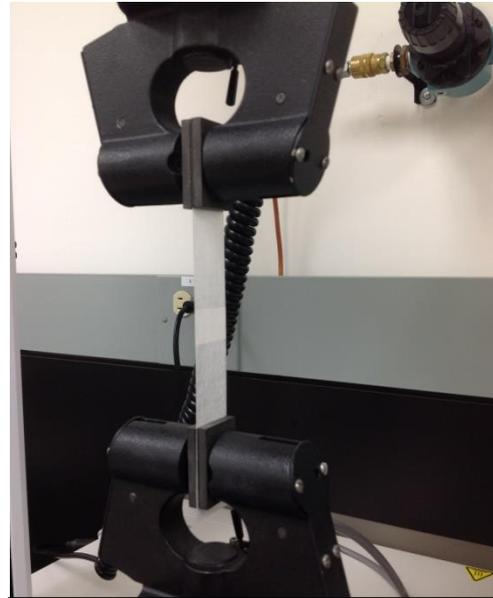
Fig. 4: LJSS sample in the tensile tester
