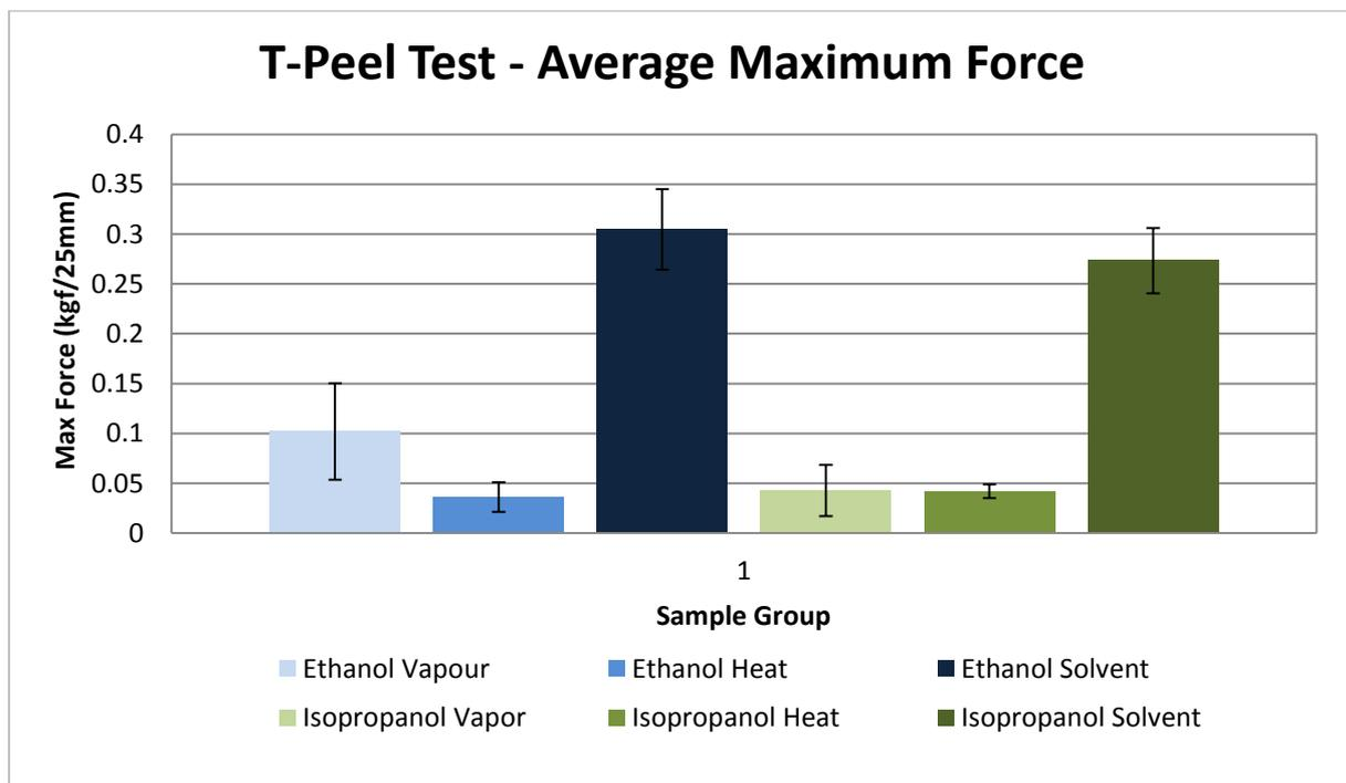
Fig. 8: T-Peel Test- Average Maximum Force
