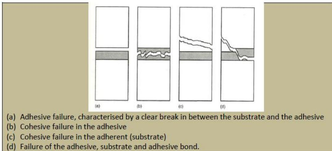
Fig. 6: Joint failure (Horie 2010)
