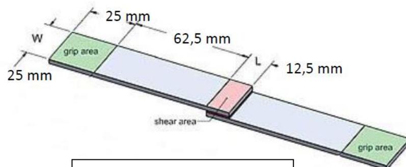
Fig. 5: LJSS sample measurements (ASTM 2010)
