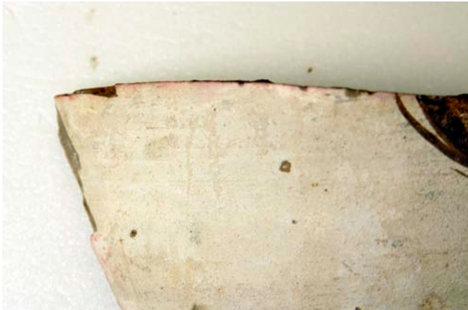
Figure 2: Stain after removal of unrefined shellac in solvent chamber (courtesy of M. Svoboda)
