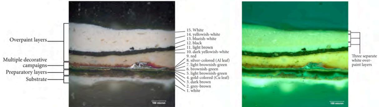
Figure 5. Example of a typical cross section, NYSS034, showing the method used for identifying and labeling the paint layers.
