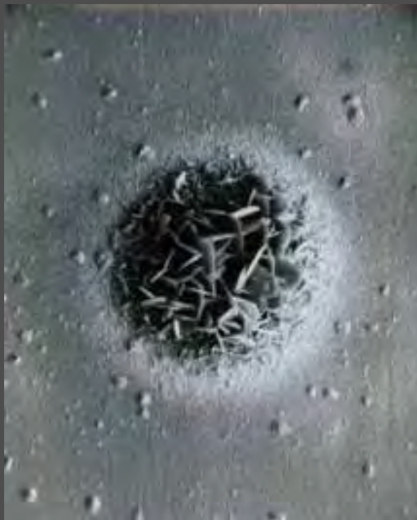
Pitting at site of high sulfur content following thiourea treatment
